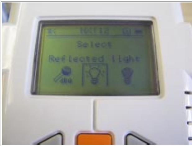
The two images above show examples of the NXT interface. Navigation is accomplished by pressing the left and right arrows and selections are made with the center, orange, button.
